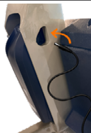
Image 13: Charging the battery in the bicycle
